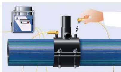
Fig 5-55: Welding the tapping fitting in accordance with DVS 2207, Part 1
