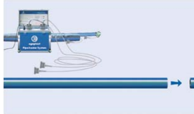
Fig 5-20: The pipe ends are prepared optimally for secure welding
