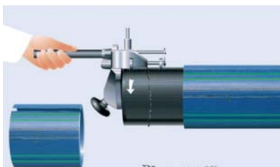
Fig 5-17: Removal of the oxide layer using a rotary scraper
