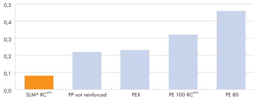
Fig 5-9: Results of scratch testing, official materials testing institute at the University of Hanover
