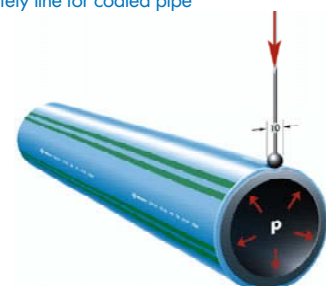
Fig 5-11: Finite element method (FEM) computational model, Muenster University of Applied Sciences, stress concentration: point and linear load safety line for coated pipe
