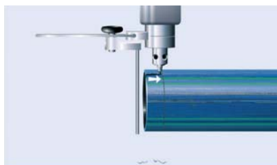
Fig 5-30: Removal of the protective coating with the egeplast coating cutter
