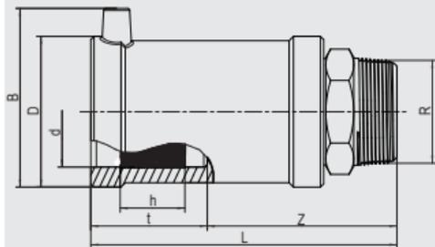
Compact transition fitting. HD-PE end with exposed heating coils for optimal heat transfer, large insertion depth, wide fusion zone plus cold zones at the end and in the transition area to prevent the flow of molten material for use without holding devices. Steel end permanently anchored in the HD-PE. Self sealing patented sealing geometry without elastomer seal. For use in gas systems.
