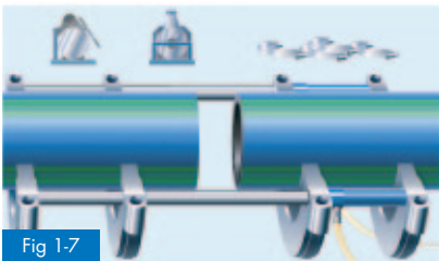
Fig 1-7 Insertion of the special clamps for protective pipes
